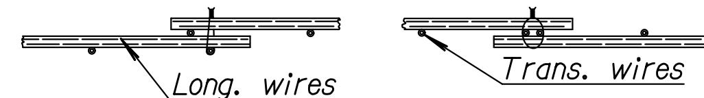
DETAIL OF LAP FOR WELDED WIRE REINFORCEMENT
